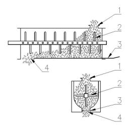
The Kiban is a steel construction fitted with a rotating shaft with steel pegs. This shaft is suspended from sturdy ball bearings. The top cover of the Kiban is equipped with clipper-de-awner cloth on the underside. Furthermore, the trough is reinforced with exchangeable steel wear plates.
