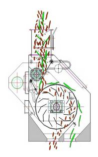
The Halmu is used for raw material such as grain or seed containing large quantities of straw or large particles that need to be removed from the material before the final treatment processes in your production line.
